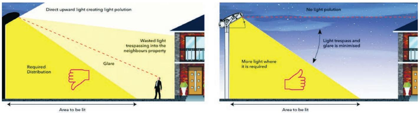
Floodlights with asymmetric distribution spread the light to where it is needed and minimise upward light spill.
